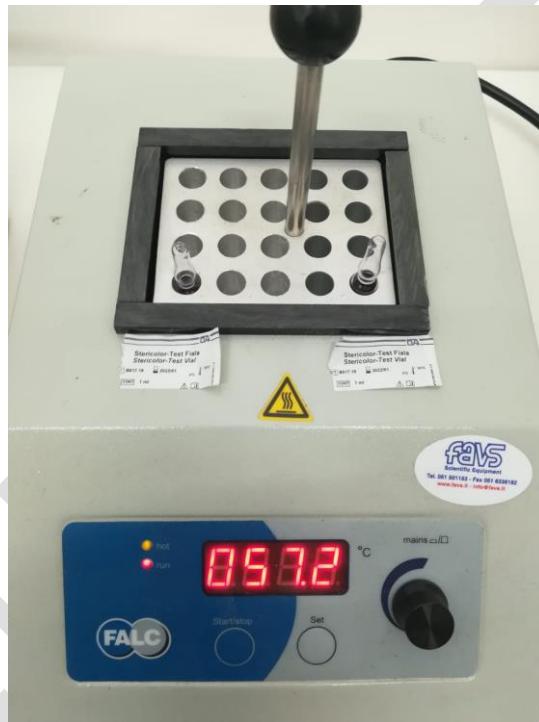
Figure 4: Vial Incubation at 55 \pm 2 °C for 48 hours
