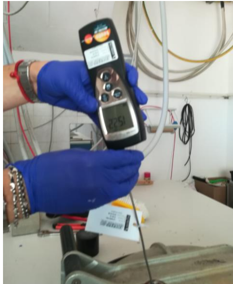
Figure 11: Temperature Measured inside the vessel
