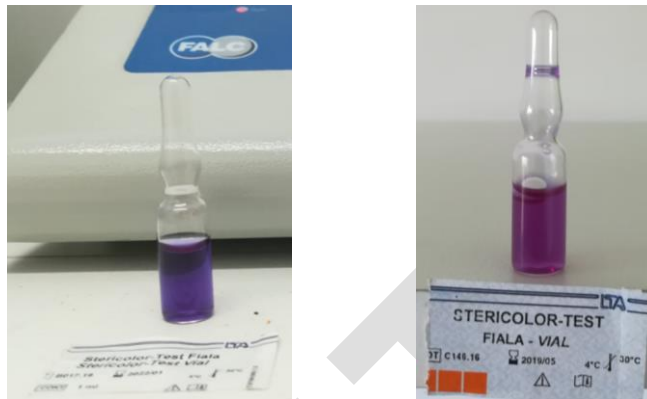
Figure 13: Bio-Indicator before incubation (on the left) and after incubation at 55-56 °C for 48 h (on the right)
