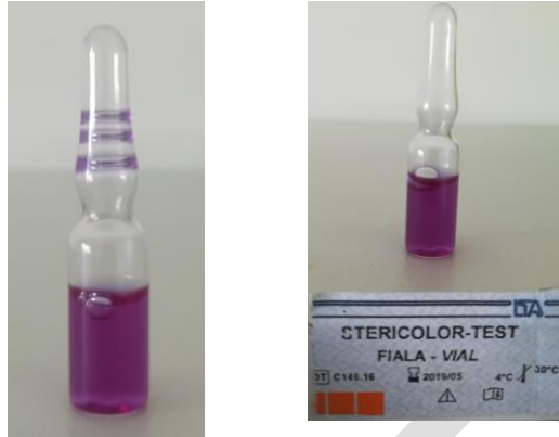
Figure 15: Bio-Indicator before incubation (on the left) and after incubation at 55-56 °C for 48 h (on the right)
