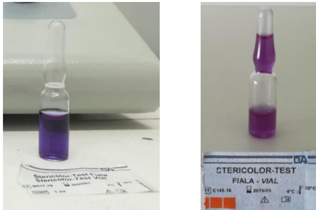
Figure 17: Bio-Indicator before incubation (on the left) and after incubation at 55-56 °C for 48 h (on the right)
