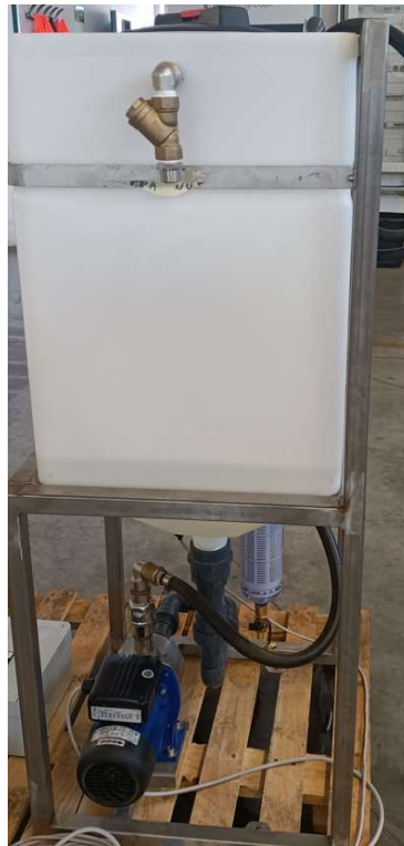
Fig. 10 Pump and water tank (optional)
