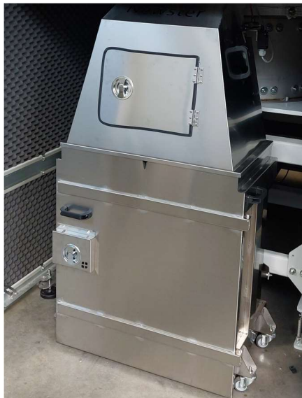
Fig. 51 - The automatic bagging system
